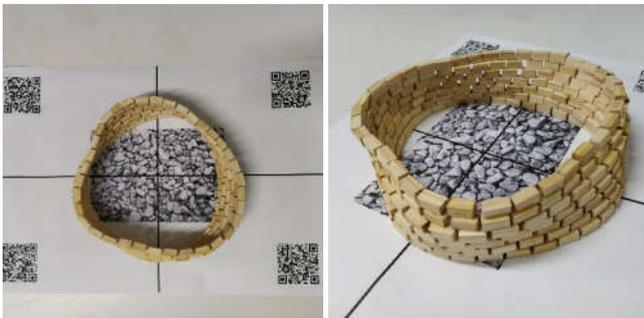
Figure 5 - prototypes assembled with AR assistance. Source: Authors.
